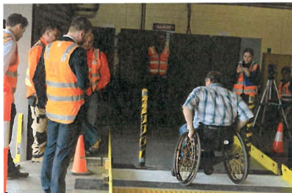
A participant traverses simulated platform gap on trial test rig
